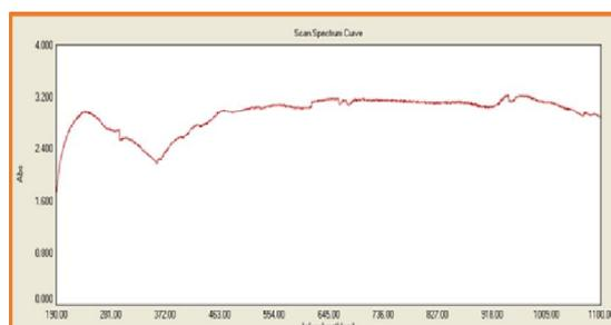
Figure 1: Scan spectrum absorption curve of the titanium dioxide nanoparticle suspension (distilled water).
